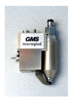
The HP glue valve can be ordered or retrofitted with an attachable 3-way easy clean valve. This valve allow the applicator to be purged of glue and cleaned with fresh water in a matter of seconds thanks to the HP's electric purge switch located directly on the gun.
